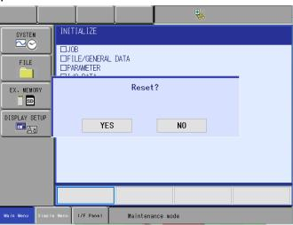
7.) Wait for the reset to complete. Once complete, the cursor on the screen will begin to move again when using the pendant up and down arrow keys.
